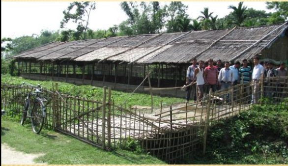
Fencing with Foot-Bath at Entrance
